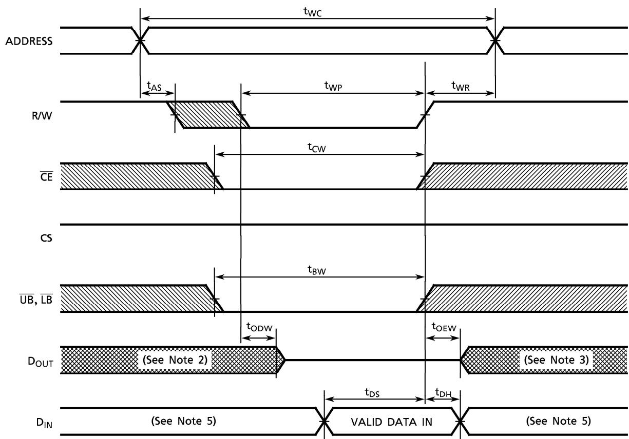
WRITE CYCLE 2 (CE CONTROLLED) (See Note 4)
