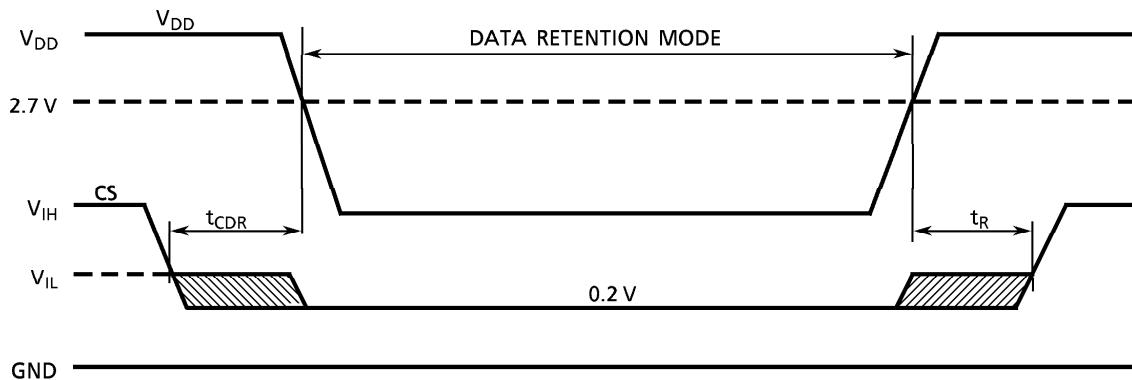
Note: (1) In  $\overline{CE}$  controlled data retention mode, minimum standby current mode is entered when  $CS \leq 0.2$  V or  $CS \geq V_{DD} - 0.2$  V.
