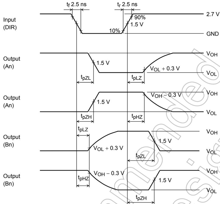
**Figure 4**  $t_{pLZ}$ ,  $t_{pHZ}$ ,  $t_{pZL}$ ,  $t_{pZH}$
