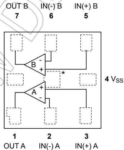
\*Central pad is not a connected pin.
