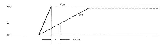
Adjust condenser value which is set  $\overline{INT}$  pin to the period while  $\overline{INT}$  pin is "L" level is longer than 1 ms when power on.
