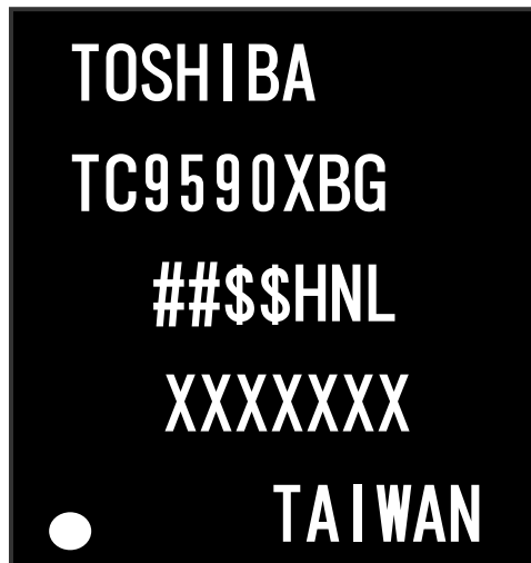
Figure 2.2 Package Marking without HDCP Key, HNL is appended to weekly code
