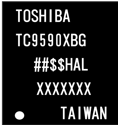
Figure 2.1 Package Marking with HDCP Key, HAL is appended to weekly code
