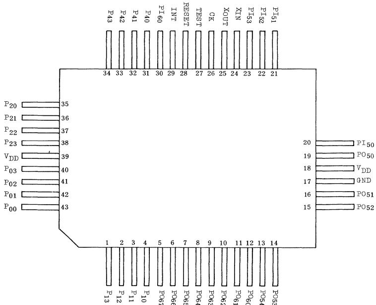
Note) Pins 18 and 39, power supply terminals, are connected in the package.
