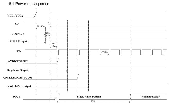
NOTE 1: RGB I/F Input → HD, DCLK, DE, R[7:0], G[7:0], B[7:0] NOTE 2: Regulator Output → VREGP, VDDP, VR, VREGN, VDDN, VMN NOTE 3: Level shifter output → STV, CKV1/2, CKH1/2/3/4/5/6, XCKH1/2/3/4/5/6, ENBV, XENBV
