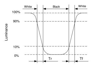
Note 10-6: Contrast Ratio in back light On (Measure System A)
