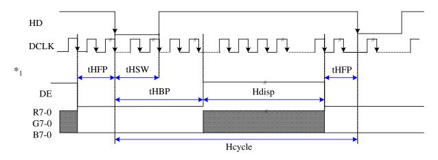
Note: The frequency of CLK should be continued whether in display or blank region to ensure IC operating normally.
