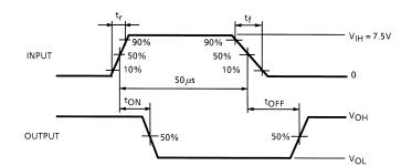
Note 1: Pulse Width 50  $\mu$ s, Duty Cycle 10% Output Impedance 50  $\Omega$ , t<sub>r</sub> ≤ 5 ns, t<sub>f</sub> ≤ 10 ns Note 2: C<sub>L</sub> includes probe and jig capacitance.
