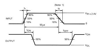
Note 1: Pulse Width 50  $\mu$ s, Duty Cycle 10% Output Impedance 50  $\Omega$ ,  $t_f \le$  5ns,  $t_f \le$  10 ns Note 2:  $C_L$  includes probe and jig capacitance
