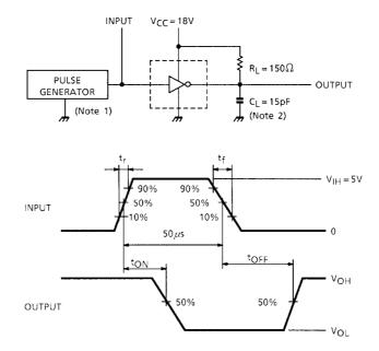
Note 1: Pulse Width 50  $\mu$ s, Duty Cycle 10% Output Impedance 50  $\Omega$ , t<sub>f</sub> ≤ 5 ns, t<sub>f</sub> ≤ 10 ns Note 2: C<sub>L</sub> includes probe and jig capacitance
