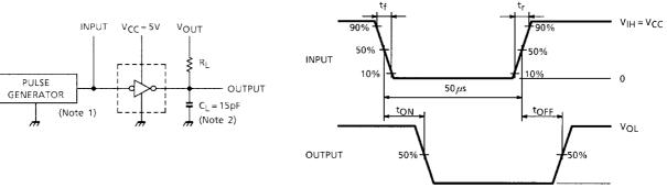
Note 1: Pulse Width 50 µs, Duty Cycle 10% Output Impedance 50  $\Omega$ , t<sub>r</sub> ≤ 10 ns, t<sub>f</sub> ≤ 5 ns Note 2: CL includes probe and jig capacitance.
