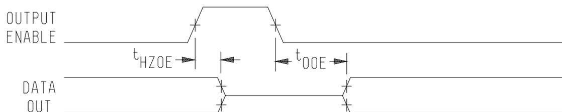
NOTE: High-Z transitions are referenced to the steady-state  $V_{OH} - 500$  mV and  $V_{OL} + 500$  mV levels on the output.
