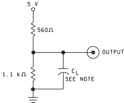
NOTE:  $C_L = 30 \text{ pF}$  and includes jig and scope capacitance.
