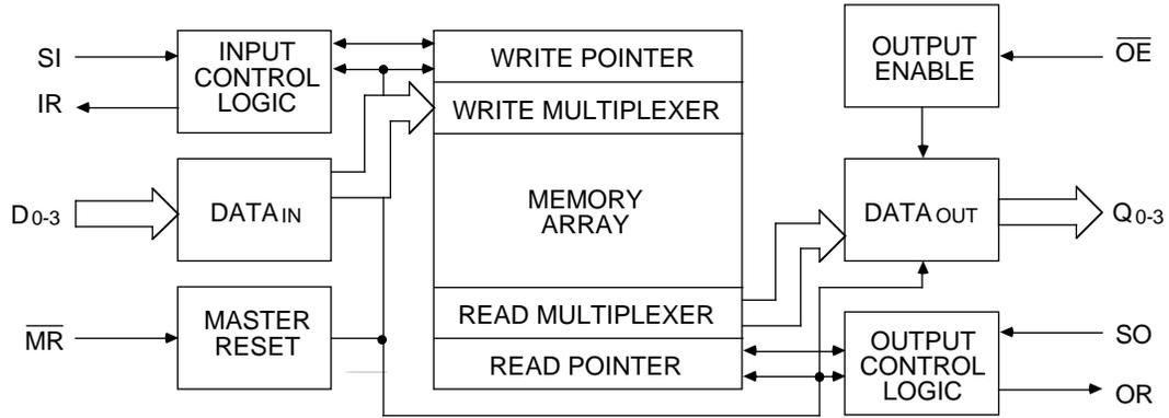
FIGURE 1. TD72403 Logic Block Diagram
