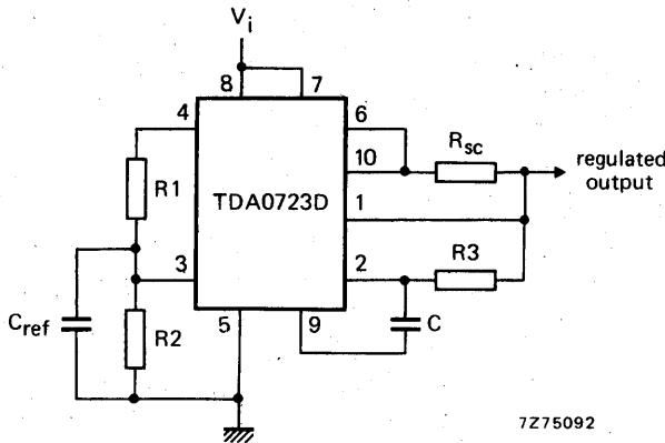
$$V_O = V_{\text{ref}} \times \frac{R_2}{R_1+R_2}$$
