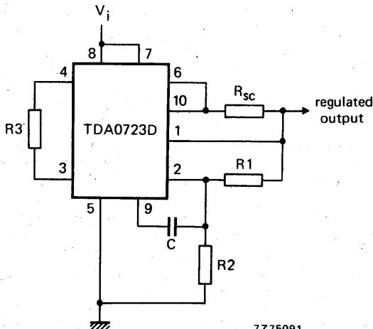
$$V_O = V_{\text{ref}} \times \frac{R_1+R_2}{R_2}$$
