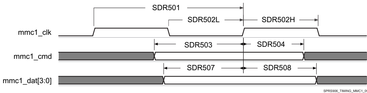
Figure 7-62. MMC/SD/SDIO in - High Speed SDR50 - Receiver Mode
