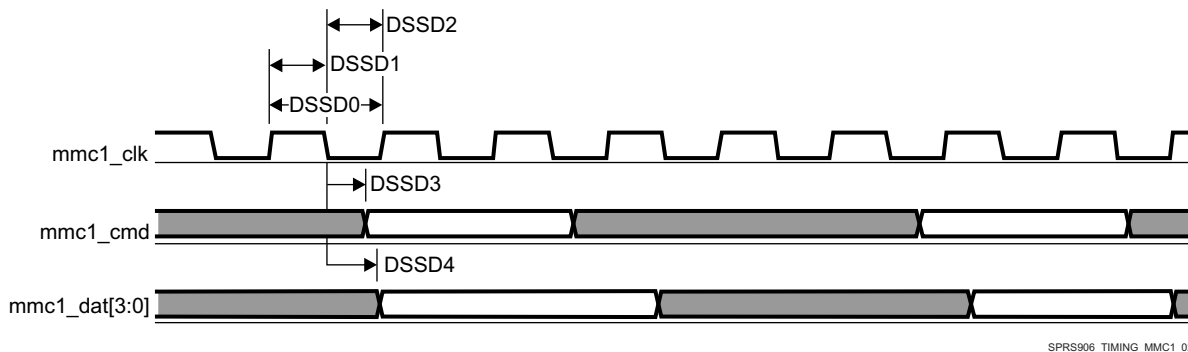
Figure 7-55. MMC/SD/SDIO in - Default Speed - Transmitter Mode
