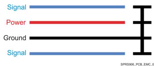
Figure 8-13. Guard Ring Routing
