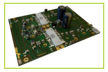
TDE800UHF is an high linear amplifier, designed to work in the entire band 470-860Mhz, with relevant power level in most common transmission standard.
