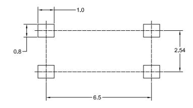
Note: All dimensions in millimeters [mm]
