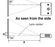
**a** (min length) = projection size (inches) × 0.04064 **a** (max length) = projection size (inches) × 0.04878
