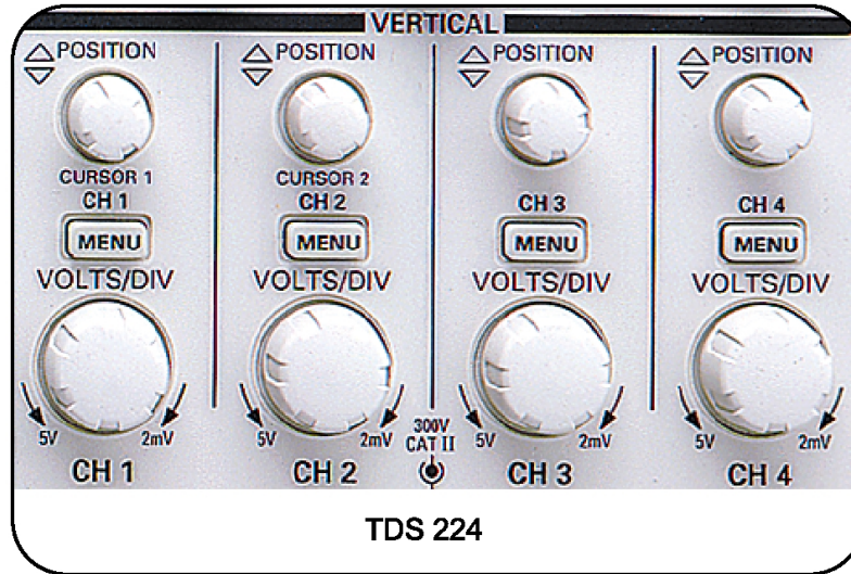
Figure 2.9: VERTICAL control knobs
