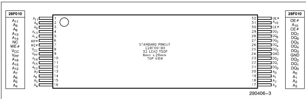
Figure 3. TSOP Lead Configuration
