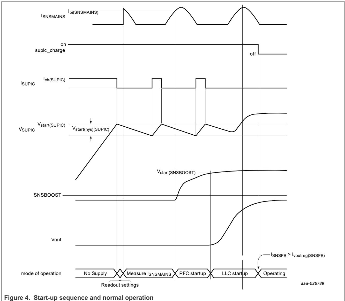
Figure 4. Start-up sequence and normal operation
