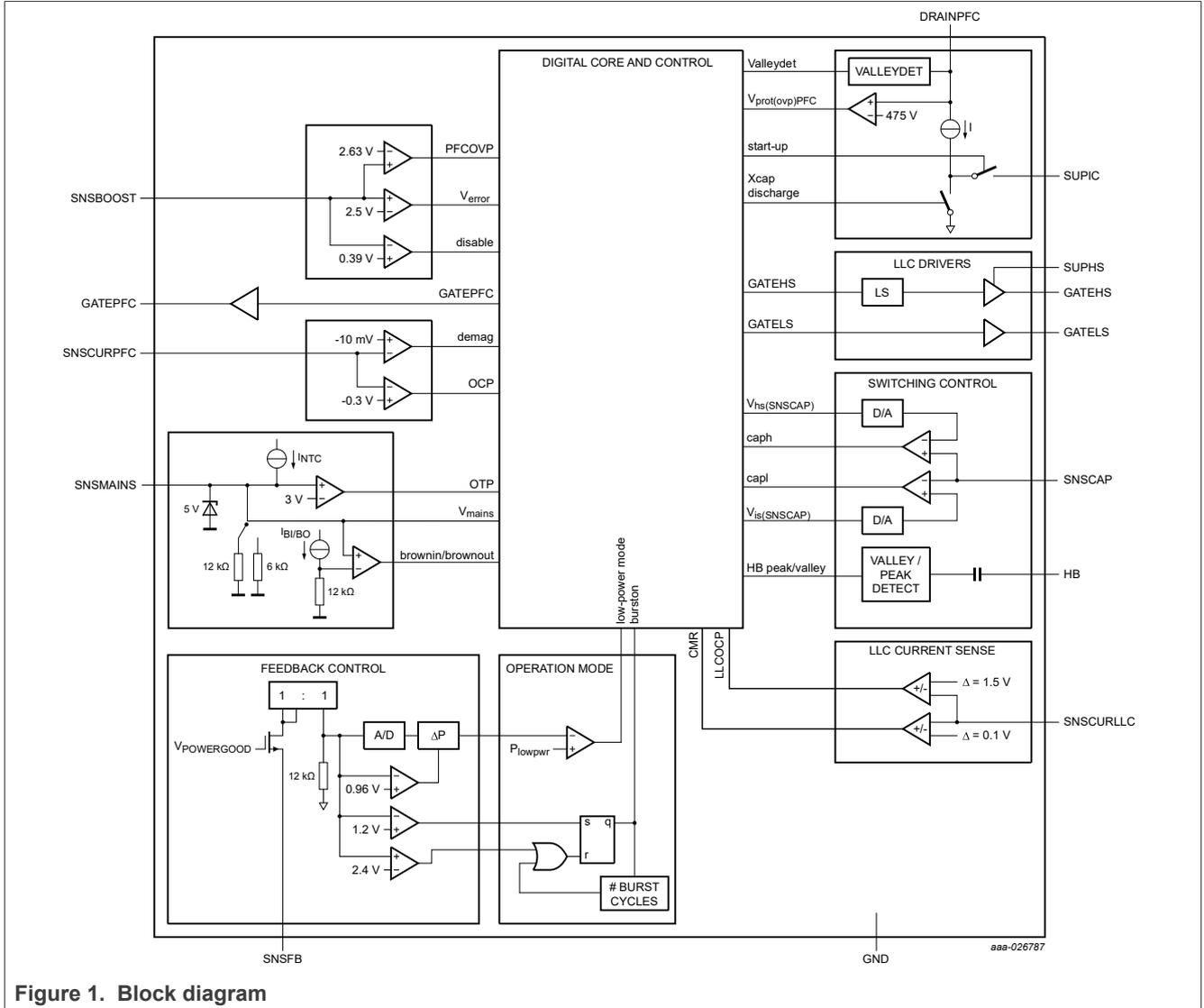
Figure 1. Block diagram
