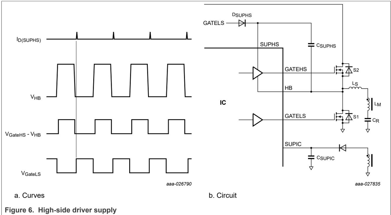
The external bootstrap buffer capacitor  $C_{SUPHS}$  supplies the high-side driver. The bootstrap capacitor is connected to the low-side driver supply, the GATELS pin, and the half-bridge node (HB) via an external diode ( $D_{SUPHS}$ ). When GATELS is active high and the HB node is pulled low,  $C_{SUPHS}$  is charged.
