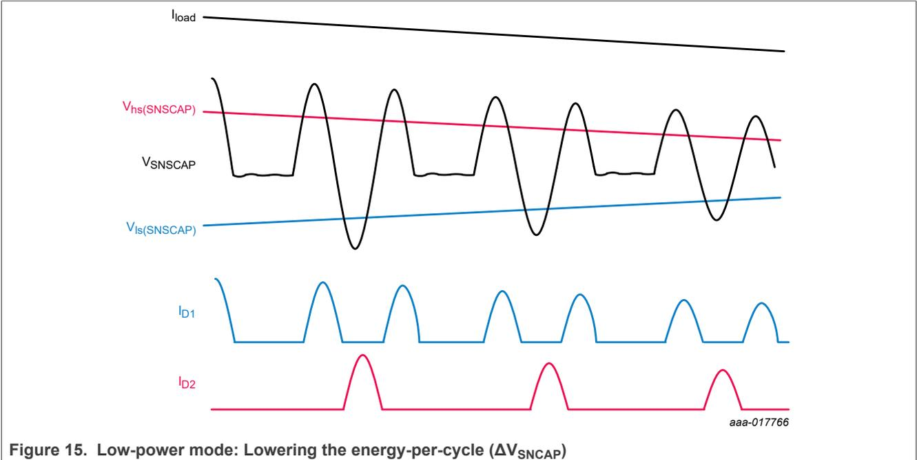
Figure 15. Low-power mode: Lowering the energy-per-cycle ( $\Delta V_{SNSCAP}$ )
