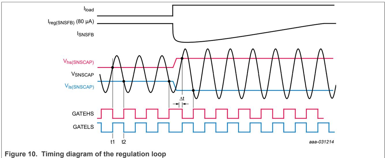
Figure 10. Timing diagram of the regulation loop
