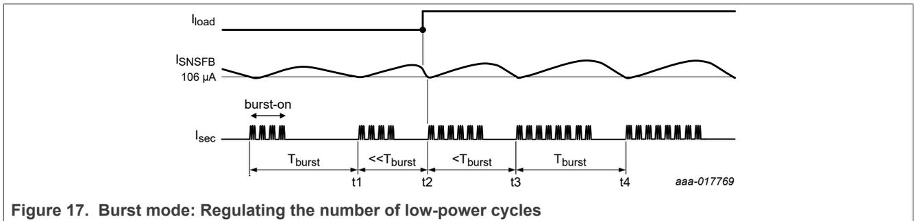
Figure 17. Burst mode: Regulating the number of low-power cycles
