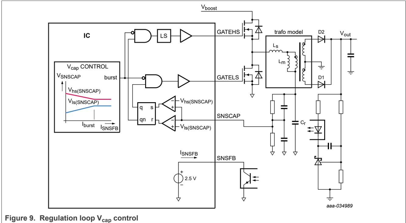
Figure 9. Regulation loop  $V_{cap}$  control
