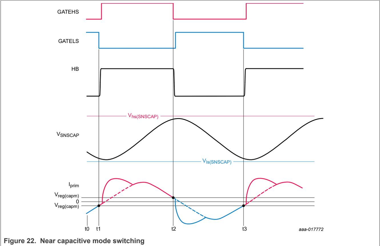
Figure 22. Near capacitive mode switching
