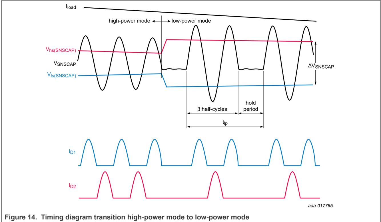
Figure 14. Timing diagram transition high-power mode to low-power mode
