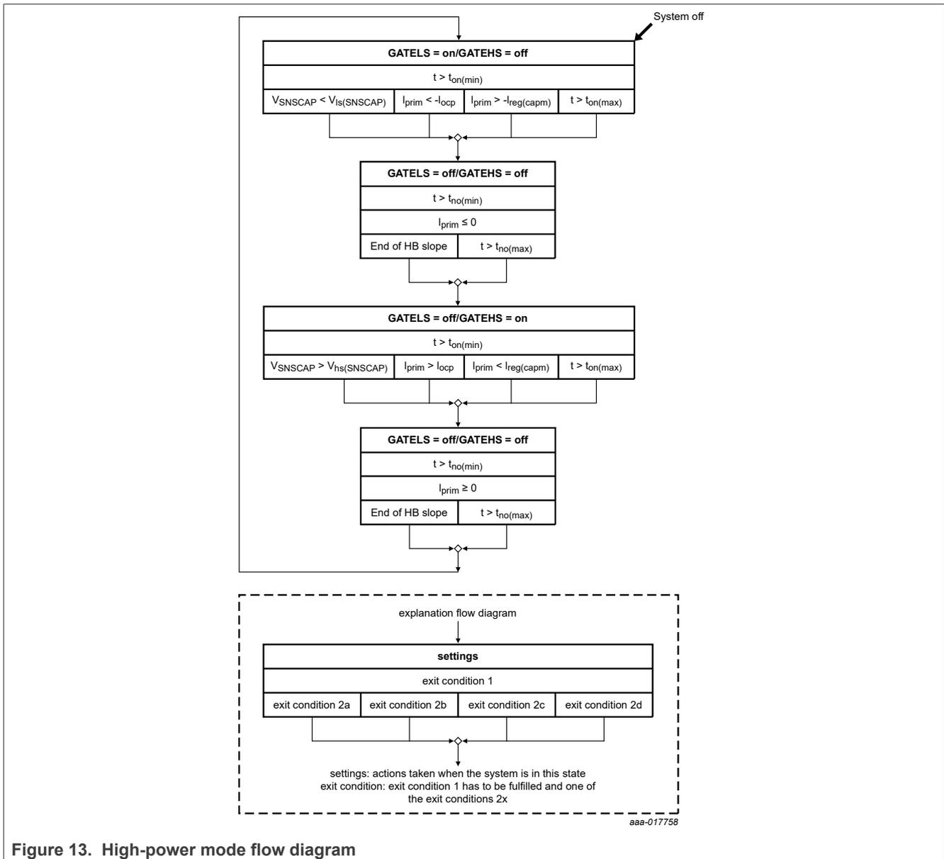
Figure 13. High-power mode flow diagram
