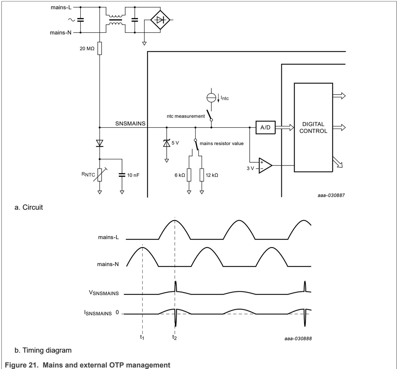
The TEA2016AAT continuously measures the SNSMAINS voltage via an A/D converter and waits until it detects a peak (t1). This peak value is internally stored and used as an input for the brownout/brownin detection and the mains compensation.
