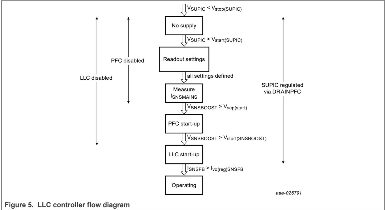
Figure 5. LLC controller flow diagram
