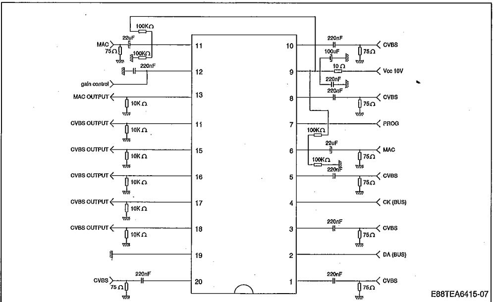
Note : When any input is not used, it must be bypassed to ground through a 220nF capacitor, so as to avoid degrading the crosstalk.
