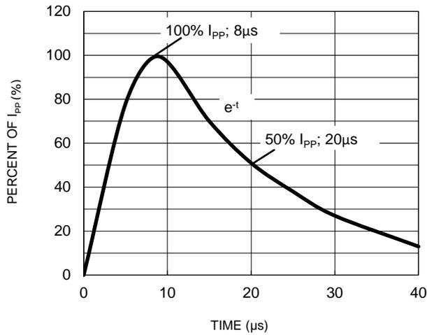
**Fig.7 ESD pulse waveform per IEC61000-4-2**
