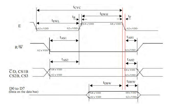
$V_{DD} = 5 \text{ V} \pm 10\%$ ;  $V_{SS} = 0 \text{ V}$ ;  $T_{amb} = -20 \text{ °C to } +75 \text{ °C}$ .
