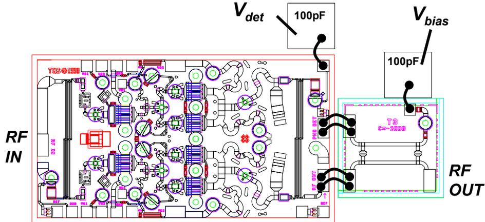
**TGA1135B with external test coupler**
