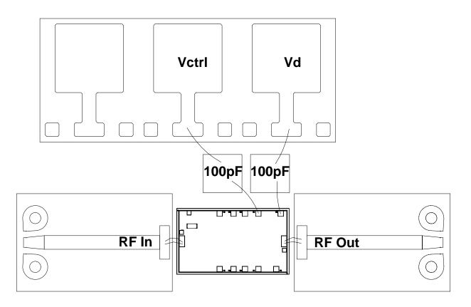
All DC connections may be brought in from either side of the chip (Use Pad 5 or 9, and Pad 6 or 8) 0.01uF external Caps are recommended on Drain line Bias: Vd = 5V (Id = ~80mA), VctrI = 0 to +5V for Gain adjustment
