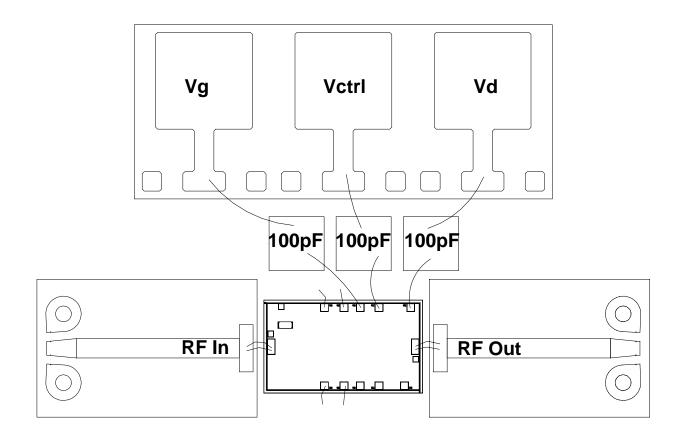
All DC connections may be brought in from either side of the chip (Use Pad 4 or 10, Pad 5 or 9, and Pad 6 or 8) 0.01uF external Caps are recommended on Drain, Gate line, 10 ohm external series R between 100pF cap and 0.01uF cap is recommended for Gate line Source connections (Pad 2, 3, 11, 12) are bonded to ground Bias: Vd = 5V, Vctrl = 0 to +5V for Gain adjustment Vg = Range, -0.5 to 0, typically ~ -0.1 will provide ~160mA of Id.
