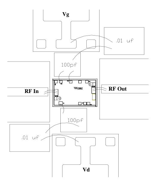
All three Vd pads (pad # 9, 10, 11 from mechanical drawing) do not need to be connected
