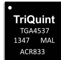
26 lead 5x5mm ACQFN package
