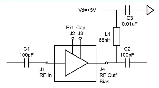
Note: Optional external capacitor can be connected between J 2 and J3 to extend functional bandwidth down to 50 MHz.
