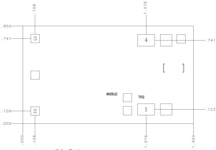
Unit: millimeters Thickness: 0.085
