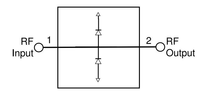
NOTE: The RF Input and RF Output ports are not interchangeable.
