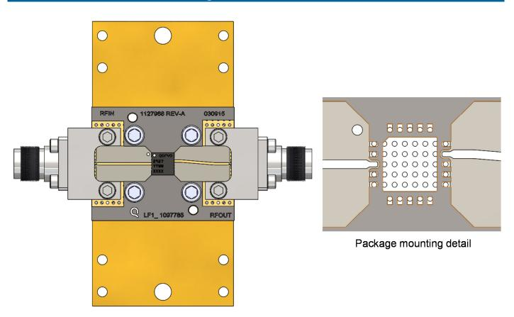
RF Layer is 0.010" thick Rogers Corp. RO4003C,  $\varepsilon_r = 3.38$ . Metal layers are 0.5 oz. copper. The microstrip line at the connector interface is optimized for the Southwest Microwave end launch connector 1092-02A-5.
