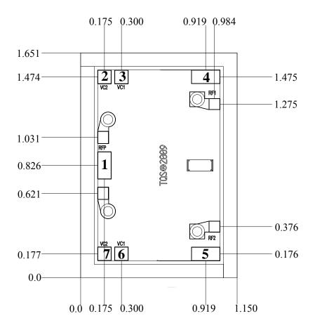
Unit: millimeters Thickness: 0.10
