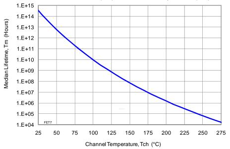
Median Lifetime (Tm) vs. Channel Temperature (Tch)
