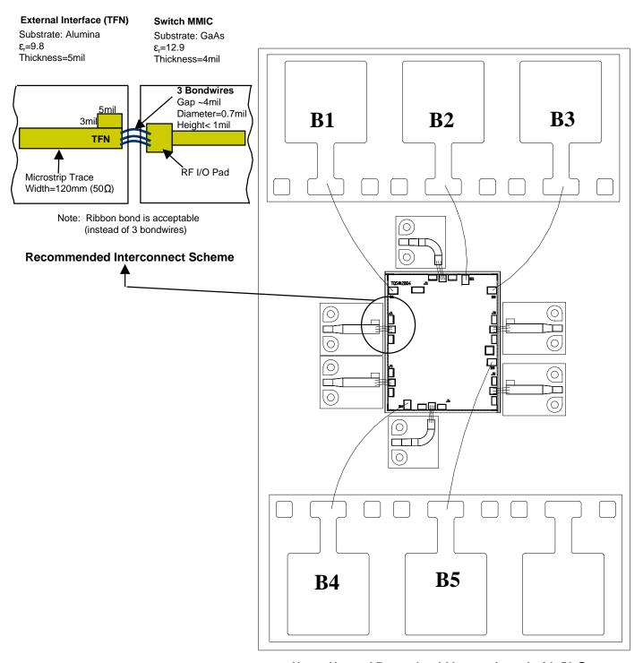
Note: Unused Ports should be terminated with 50  $\Omega$ .
