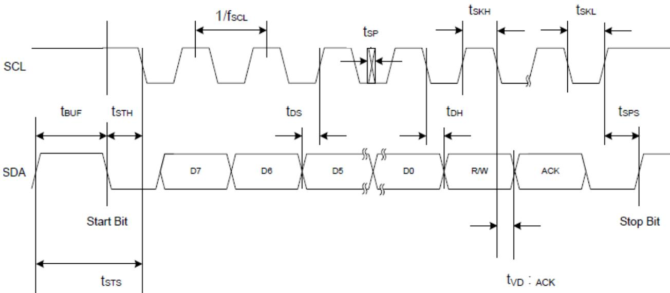
**Figure 1. I<sup>2</sup>C Interface Timing Diagram**
