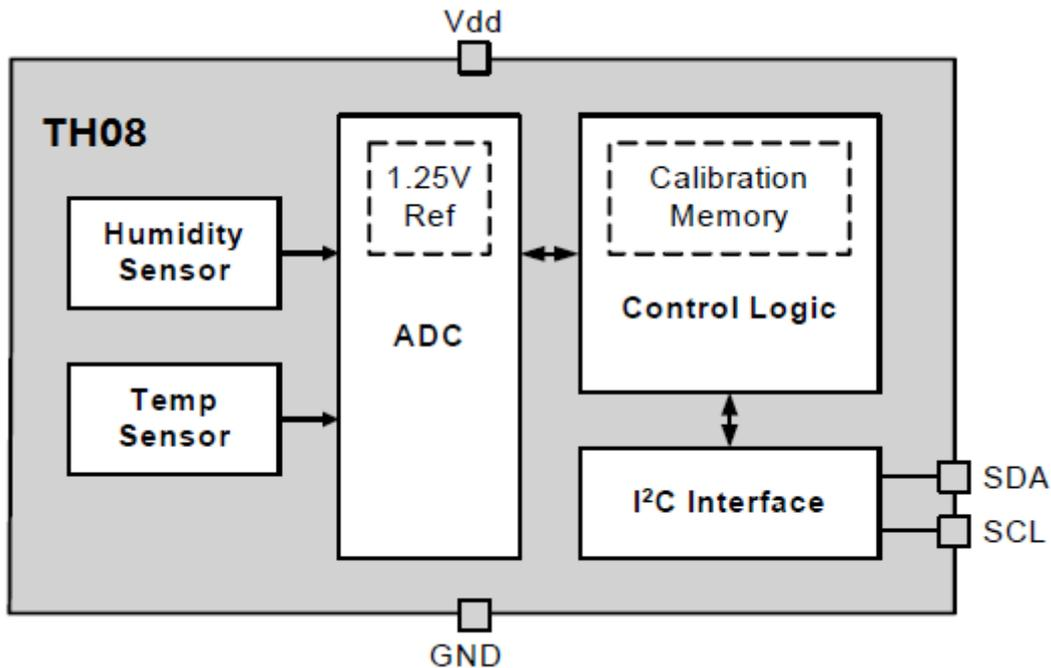
**Figure 5. TH08C Block Diagram**
