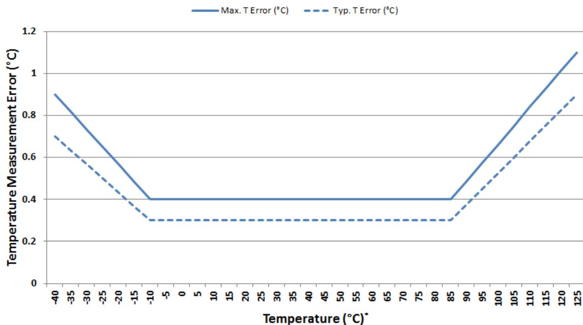
Figure 3. Temperature Accuracy
