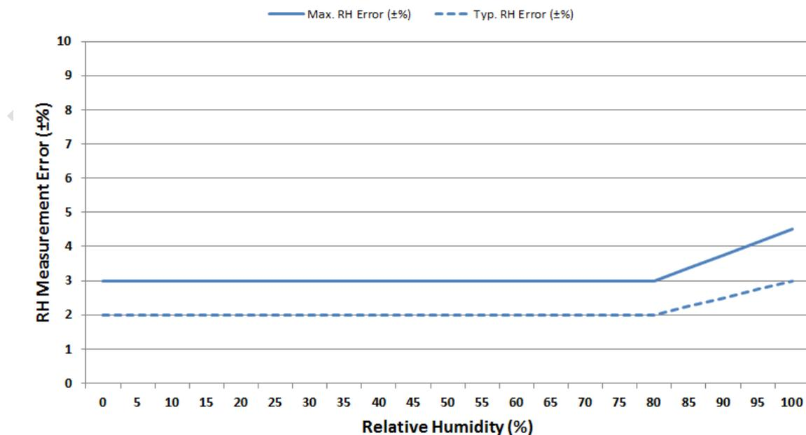
Figure 2. RH Accuracy at 30 °C
