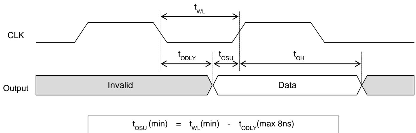
**Figure 2 Output timing**
