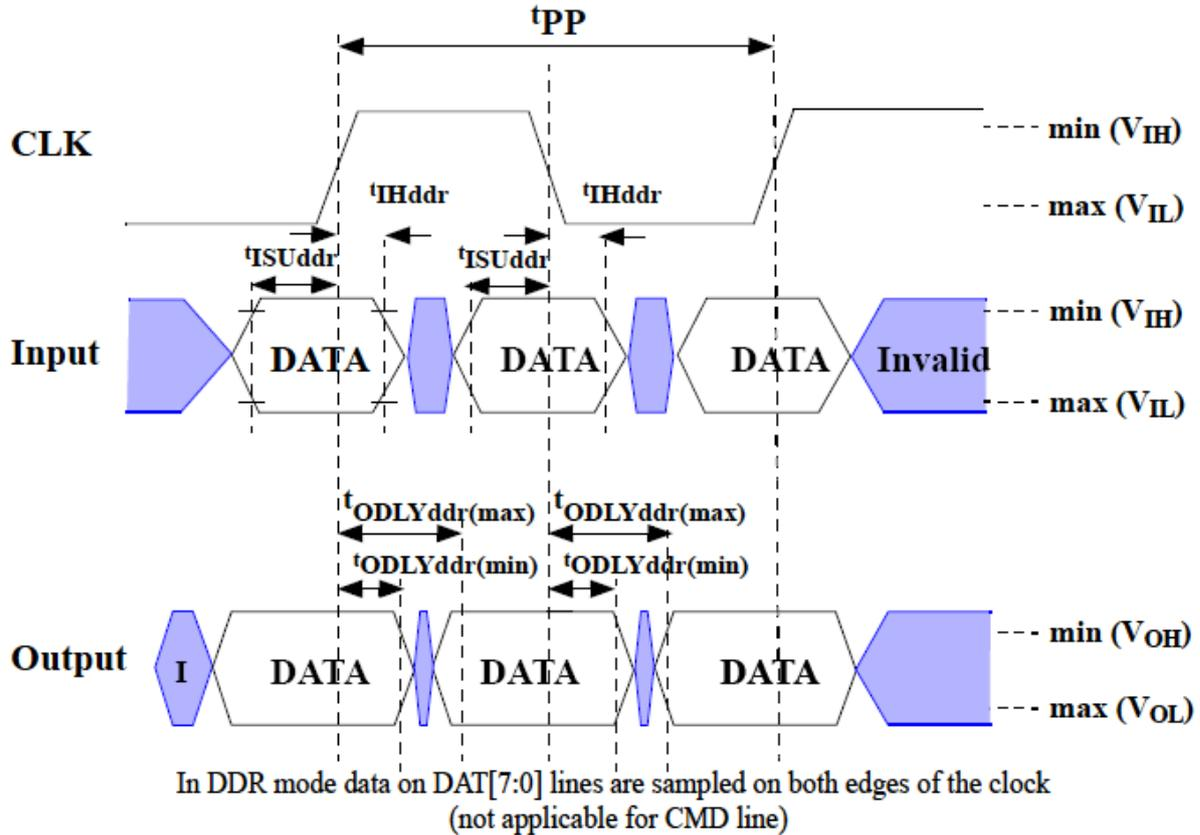
**High-speed dual data rate interface timings**
