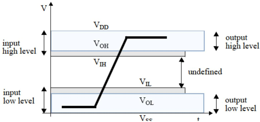
**Open-Drain Mode Bus Signal Level**
