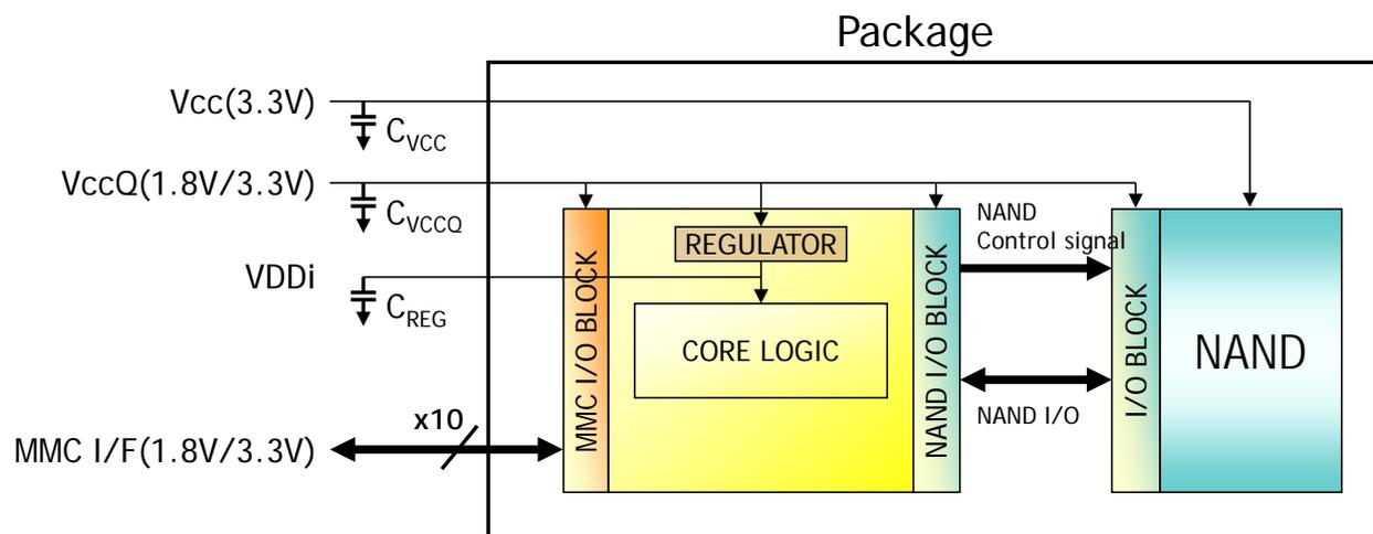
Figure 1 THGBM5G5A1JBAIR Block Diagram
