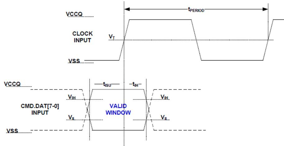
Note1:  $t_{ISU}$  and  $t_{IH}$  are measured at  $V_{IL(max)}$  and  $V_{IH(min)}$ .
