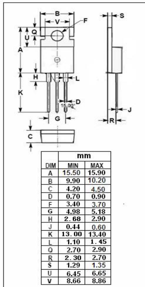
**isc N-Channel MOSFET Transistor****TK10E80W, ITK10E80W****ELECTRICAL CHARACTERISTICS****T<sub>C</sub>=25°C unless otherwise specified**
