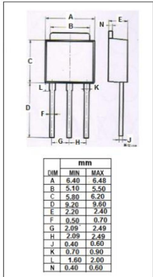
**isc N-Channel MOSFET Transistor****TK10Q60W, ITK10Q60W****ELECTRICAL CHARACTERISTICS**T<sub>C</sub>=25°C unless otherwise specified
