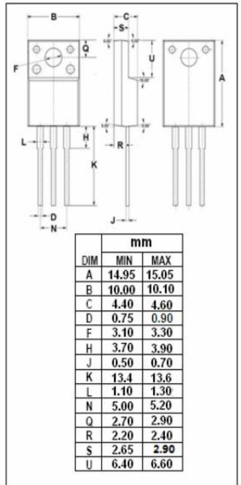
**iscN-Channel MOSFET Transistor****TK13A65U, ITK13A65U****ELECTRICAL CHARACTERISTICS**T<sub>C</sub>=25°C unless otherwise specified
