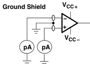
Figure 5. Input Bias and Offset Current Test Circuit
