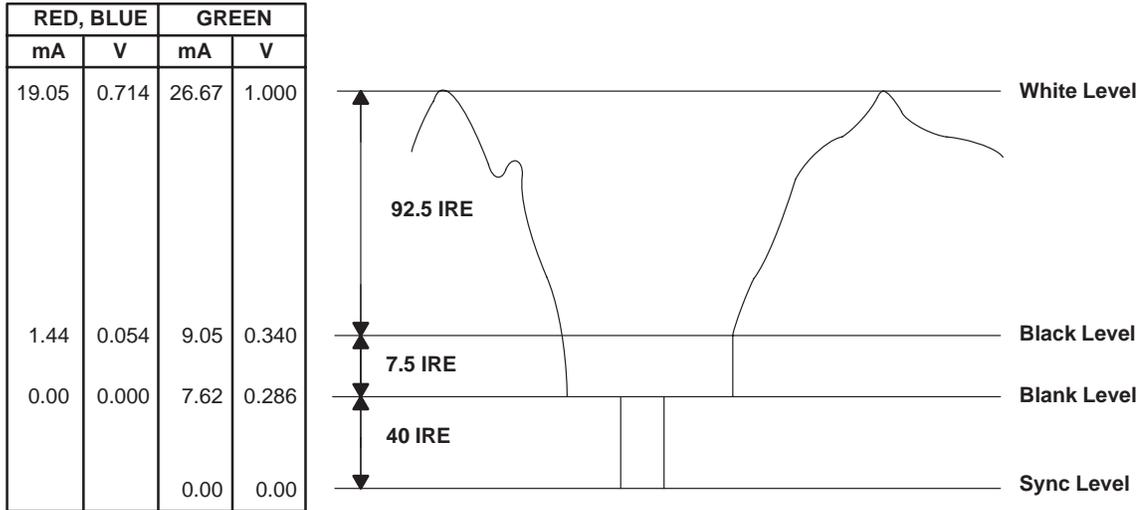
NOTE A: The IRE (Institute of Radio Engineers – now IEEE) scale is used for defining the relative voltage levels of the sync, white, black, and blank levels in a monitor circuit. The reference white level is set at 100 IRE units. The blanking level is set at  $\phi$  IRE units. One IRE unit is equivalent to 1/100 of the difference between the reference white level and the blanking level.
