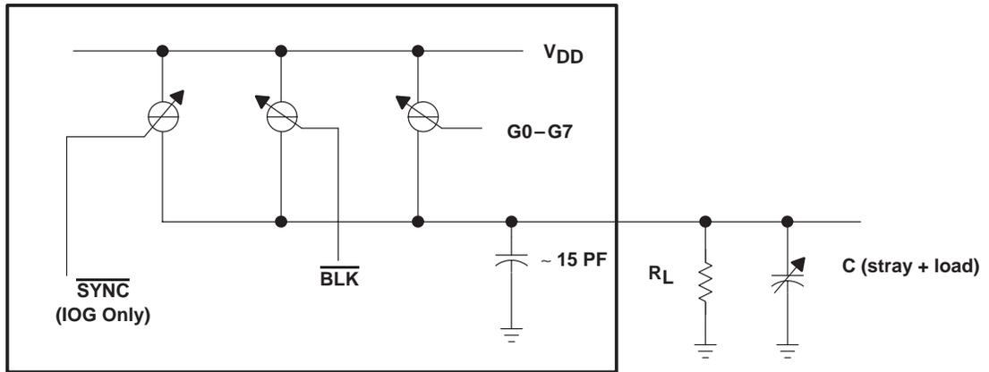
Figure 6. Equivalent Circuit of the Current Output (IOG)
