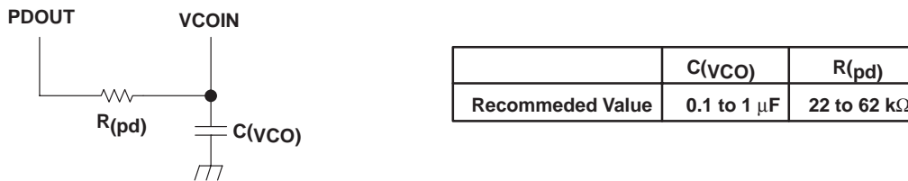
Figure 8. Resistor and Capacitor Connection
