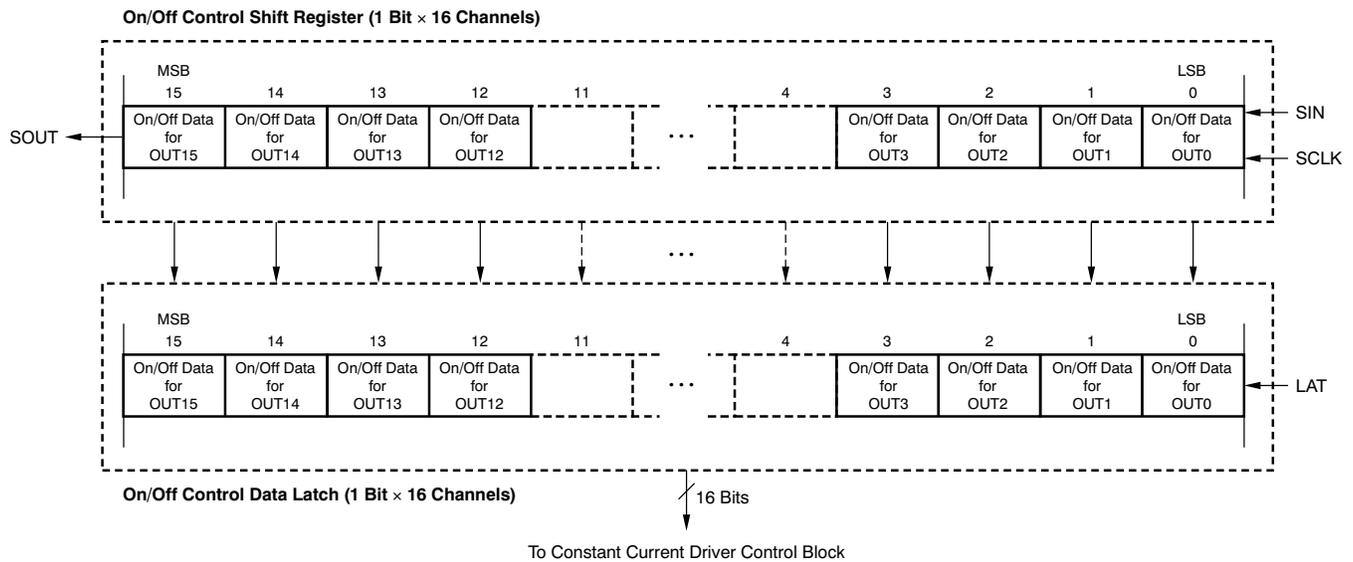
**Figure 17. On/Off Control Shift Register and Latch Configuration**
