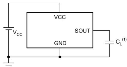
(1)  $C_L$  includes measurement probe and jig capacitance.
