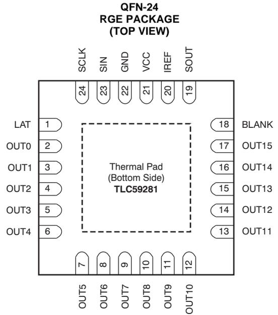
NOTE: Thermal pad is not connected to GND internally. The thermal pad must be connected to GND via the PCB pattern.
