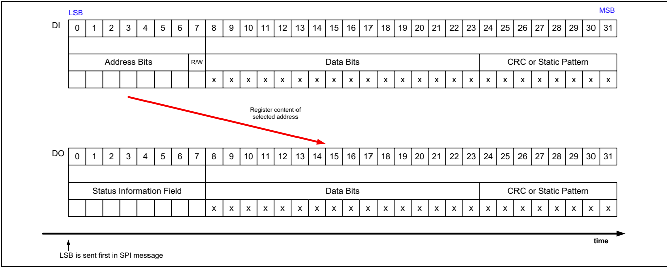
Figure 76 SPI Operation Mode
