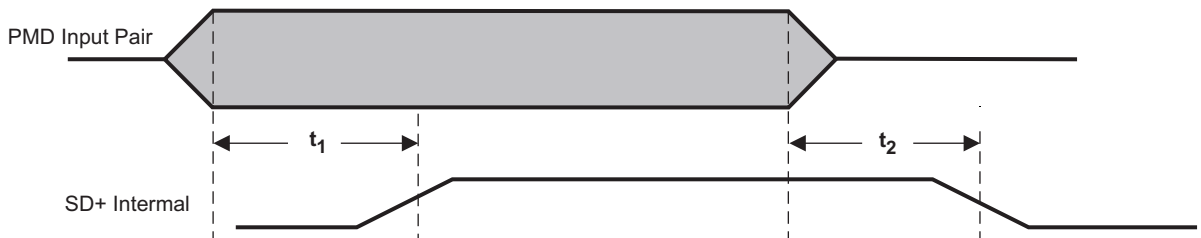
Figure 9-20. 100BASE-TX Signal Detect Timing
