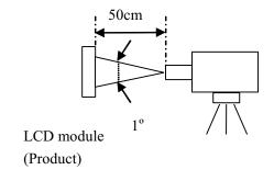
Luminance Meter (TOPCON BM-5A) Spectroradiometer(TOPCON SR-3)
