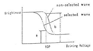
Contrast Ratio =  $b / a = \frac{\text{non-selected state brightness}}{\text{selected state brightness}}$
