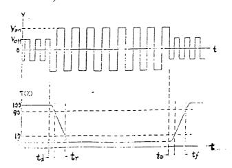
Turn-on time:  $t_{on} = t_d + t_r$
