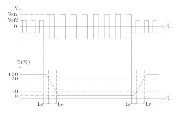
Turn on time:  $t_{on} = t_d + t_r$  Tur Measuring Condition: 1) Operating Voltage: 6.5V
