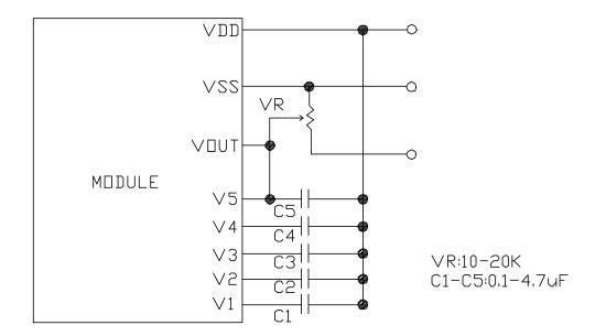
Both the boosting circuit and the voltage control circuit are not used in this module.
