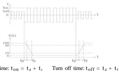
Turn on time:  $t_{on} = t_d + t_r$  Tu Measuring Condition:
