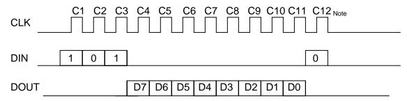
The DIN data in C1 $\sim$ C3 cycle is R08 command, C1 is MSB, C3 is LSB. The DOUT data in C4 $\sim$ C11 cycles are the output data from Register 08, D7 = R08 $_{\circ}$ , D6 = R08 $_{\circ}$ , ......D0 = R08 $_{\circ}$ .
