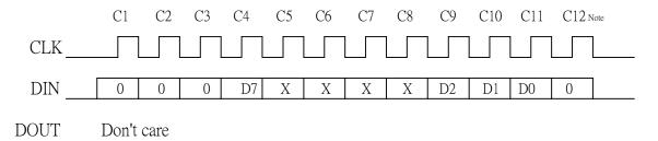
The DIN data in C1~C3 cycle is STCH command, C1 is MSB, C3 is LSB. The DIN data in C4 cycle is Oscillator enable bit, D7=ENOSC. The DIN data in C5~C8 cycle don't care. The DIN data in C8~C10 cycle is A/D converter (comparator) channel selection information, D2 = CHSEL2, D1 = CHSEL1, D0 = CHSEL0.
