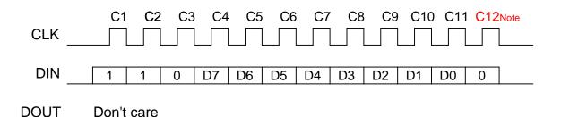
The DIN data in C1~C3 cycle is WR9 command, C1 is MSB, C3 is LSB. The DIN data in C4~C11 cycles are the input data for Register 09, D7 =  $R09_7$ ,
