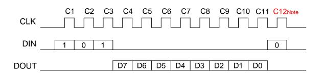
The DIN data in C1~C3 cycle is R08 command, C1 is MSB, C3 is LSB. The DOUT data in C4~C11 cycles are the output data from Register 08, D7 = R08<sub>7</sub>, D6 = R08<sub>6</sub>,... D0 = R08<sub>0</sub>.
